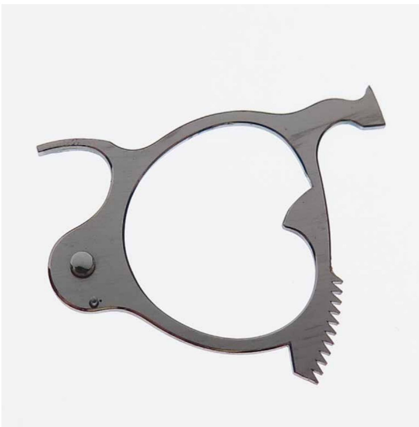
The small snail on top of the hour rack drives the 5 minute rack shown below.
